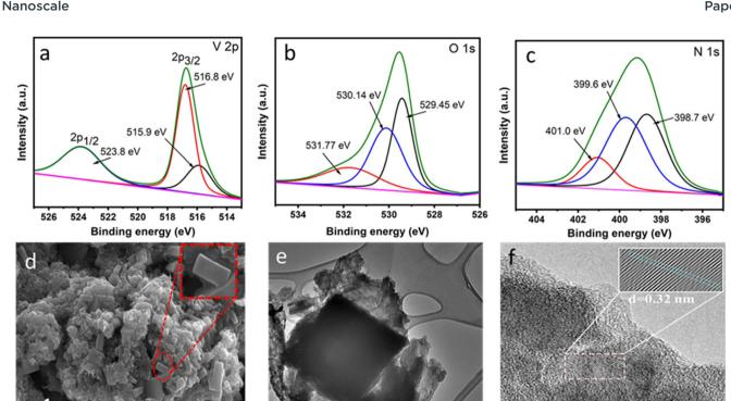
Fig. 3 XPS spectra of VO<sub>2</sub>@CN: (a) V 2p, (b) O 1s and (c) N 1s. (d) FESEM image of VO<sub>2</sub>@CN indicating the presence of blocks of VO<sub>2</sub> encapsulated in crumpled N-doped C layers. TEM and HRTEM images of VO2@CN are presented as (e) and (f), respectively.
