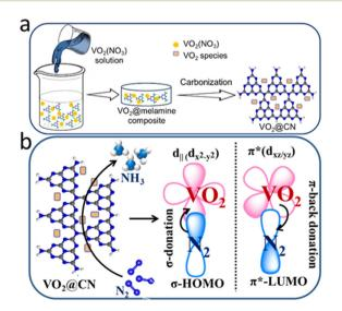
Fig. 1 (a) Schematic representation of the synthesis of VO2@CN; (b) orbital interaction between N2 and the VO2 centre of the catalyst, responsible for  $N_2$  reduction to  $NH_3$  (NRR).
