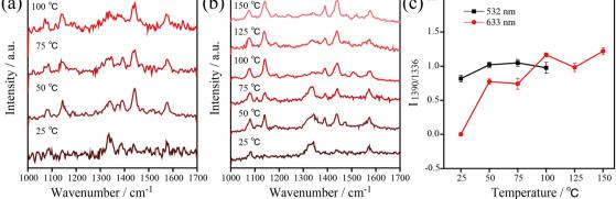
Fig. 5 Temperature-dependent SERS spectra of the plasmon-induced photocatalytic reaction of 4-NTP at high temperatures with 532 nm (a) and 633 nm (b) excitation, respectively,  $t_{acq} = 60$  s. (c) intensity ratio of 1390 cm<sup>-1</sup>/1336 cm<sup>-1</sup> referring to [DMAB]/[4-NTP] as a function of temperature at 532 nm (black) and 633 nm (red) ( $P_{532 \text{ nm}} = 1.05 \text{ µW}$ ,  $P_{633 \text{ nm}} = 7.8 \text{ µW}$ ).
