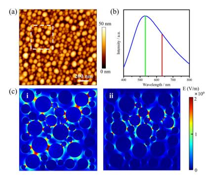
Fig. 2 (a) AFM topography image and (b) normalized extinction spectrum of AgNIs; (c) simulated electric field distribution of AgNIs (a 300 x 300 nm<sup>2</sup> region extracted from the AFM image) under 532 nm (i) and 633 nm (ii) excitation, respectively.
