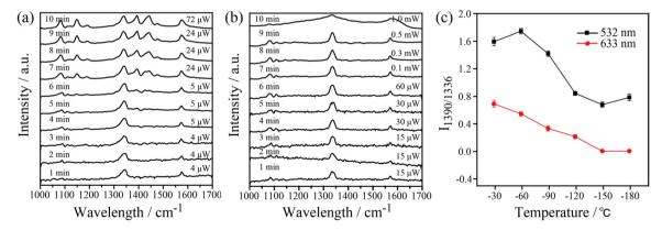
Fig. 4 Time-dependent SERS spectra of the plasmon-induced catalytic reaction of 4-NTP at -180 °C with (a) 532 nm and (b) 633 nm excitation at different laser powers on the samples. The time interval is 1 min from bottom to top,  $t_{acq} = 60 \text{ s}$ ; (c) the average intensity ratio of 1390 cm<sup>-1</sup>/ 1336 cm<sup>-1</sup> referring to [DMAB]/[4-NTP] as a function of temperature at 532 nm (black) and 633 nm (red).
