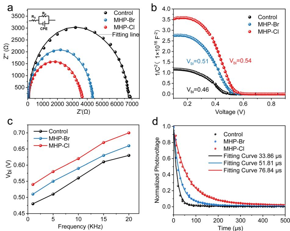
**Fig. 4** (a) Nyquist plots (inserted picture is the equivalent circuit model). (b) The Mott-Schottky plot of capacitance versus voltage measured under 1 kHz. (c) The extracted  $V_{bi}$  values of the CQD devices under different frequencies. (d) Photovoltage decay spectra of the CQD solar cells.
