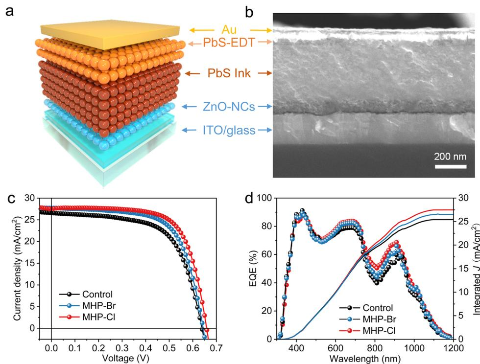
**Fig. 3** (a) Schematic illustration of the CQD photovoltaic device. (b) Cross-section SEM image of the PbS CQD photovoltaic device used in this study. (c)  $J$ - $V$  curves of CQD solar cells obtained under an AM 1.5G solar simulator. (d) EQE curves and integrated JSC of the best devices.
