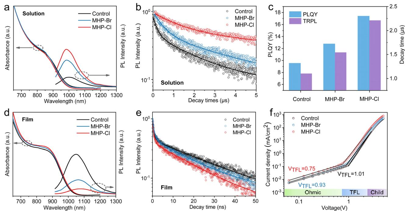
**Fig. 2** (a) Absorbance and steady-state PL spectra of PbS QD solutions. (b) TRPL of the QD inks. (c) PLQY and TRPL results of the QD solutions. (d) Absorbance and steady-state PL spectra of the QD solid films. (e) TRPL of the QD films. (f) Space charge limited current (SCLC) measurements for the QD films.
