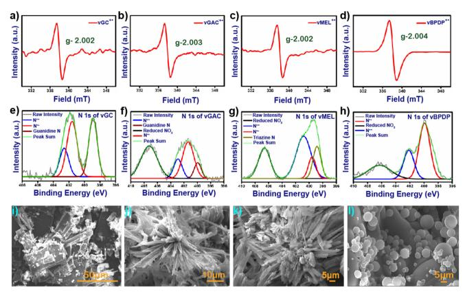
Fig. 2 Solid-state EPR spectra of (a) vGC, (b) vGAC, (c) vMEL and (d) vBPDP in the radical cationic state. N 1s XPS spectra of (e) vGC, (f) vGAC, (g) vMEL and (h) vBPDP. FE-SEM micrographs of (i) vGC, (j) vGAC, (k) vMEL and (l) vBPDP.
