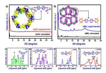
**Fig. 3** Comparison of experimental PXRD pattern with the simulated powder pattern of (a) vGAC and (b) vMEL. Solid-state <sup>13</sup>C CP-MAS NMR spectra of (c) vGC, (d) vGAC, (e) vMEL and (f) vBPDP.
