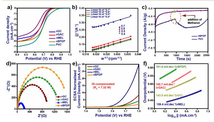
Fig. 4 (a) LSV curves of all vCONs, (b) K-L plot of vBPDP, (c) methanol stability of vBPDP, (d) EIS spectra of all vCONs, (e) LSV curves for the OER of all vCONs, and (f) Tafel plots of all the vCONs.
