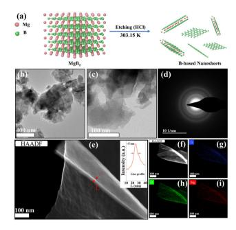
Fig. 1 (a) Schematic illustration for the preparation of boron-based nanosheets. (b) TEM image of  $MgB_2$ . (c) TEM image of Mg-BNSs. (d) SAED pattern of Mg-BNSs. (e) HAADF of a thin nanosheet. The inset image is the line profile at position "L". (f–i) EDS mappings of a thin nanosheet.
