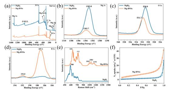
Fig. 2 XPS spectra of (a) survey, (b) Mg 1s, (c) O 1s, and (d) B 1s of MgB<sub>2</sub> and Mg-BNSs. (e) Raman spectra of MgB<sub>2</sub> and Mg-BNSs. (f) N<sub>2</sub> adsorption—desorption curves of MgB<sub>2</sub> and Mg-BNSs.
