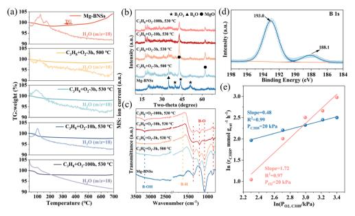
Fig. 4 (a) TG-MS analysis of Mg-BNSs and their spent forms under an  $O_2$ -rich atmosphere (20%  $O_2$  + 80%  $N_2$ ). (b) XRD patterns and (c) FT-IR spectra of Mg-BNSs and the spent Mg-BNSs activated in the reaction atmosphere at different temperatures and durations. (d) B 1s XPS spectrum of Mg-BNSs tested for 100 h over ODHP. (e) Reaction rate as a function of the partial pressure of propane and oxygen in ODHP over Mg-BNSs. The data were obtained at 480 °C.
