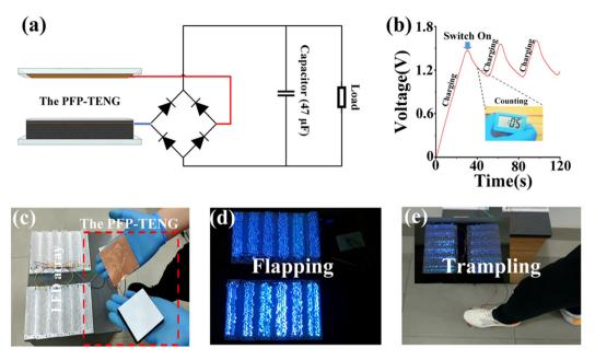
Fig. 5 Application of PFP-TENG to drive low-power loads. (a) Using an external circuit drives (b) the electronic clock. (c) The PFP-TENG is applied in different motion occasions, such as (d) flapping and (e) trampling.
