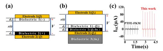
Fig. 2 The theoretical model of PFP: (a) the traditional vertical contact-separated TENG, (b) the PFP-TENG. (c) The comparison of  $I_{SC}$  between (d) PTFE-PU TENG and (e) PTFE-FKM TENG with PU substrate. (f) The effect of PU on  $I_{SC}$ .
