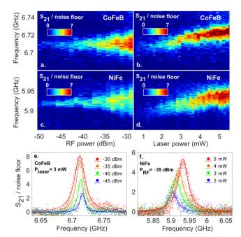
Fig. 3 Typical spectra vs.  $P_{RF}$  and  $P_{laser}$  of CoFeB (a) and (b) at  $I_{DC}$  = 0.65 mA, and NiFe (c) and (d) at  $I_{\rm DC}$  = 3.4 mA. The colorbar scale represents the measured S<sub>21</sub> normalized over the average noise floor level. The left column measurements were performed at fixed  $P_{laser}$  = 3 mW, while the right column measurements at  $P_{RF} = -35$  dBm. Two-dimensional spectra with lorentizian fittings (solid lines) are shown for CoFeB (e) and NiFe (f).
