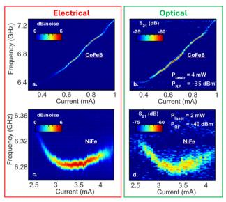
Fig. 2 Typical power spectral density (PSD) vs. I<sub>DC</sub> measurements of CoFeB (a) and (b) and NiFe (c) and (d) SHNOs. The left column (a) and (c) shows traditional electrical measurements and the right column (b) and (d) shows the corresponding optical measurements. The applied field conditions were H=3600 Oe,  $\theta=65^{\circ}$ , and  $\phi=22.5^{\circ}$  for CoFeB and H = 6300 Oe,  $\theta$  = 82°, and  $\phi$  = 22.5° for NiFe.
