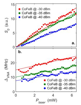
Fig. 5 Extracted (a)  $S_0$  and (b)  $\Delta_{VNA}$  vs.  $P_{laser}$  for the CoFeB SHNO. Solid lines represent linear fits to the data. The intercepts with  $P_{laser} = 0$  of the fits in b. are shown as pale blue stars in Fig. 4b and used to extract the intrinsic free-running SHNO linewidth ( $\Delta f$ ).
