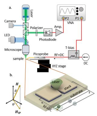
Fig. 1 (a) Schematic of the experimental setup: red lines represent electrical connections. Green lines represent the laser path. In blue, the LED illumination light path. (b) Zoom view of the sample (substrate and stack) and reference axes. The SHNO is subject to an external DC+RF stimulus. The external magnetic field H, its polar  $(\theta)$  and azimuthal  $(\phi)$  field angles, and its in-plane component  $H_{\rm IP}$  are shown. The incident laser probe is shown in green.
