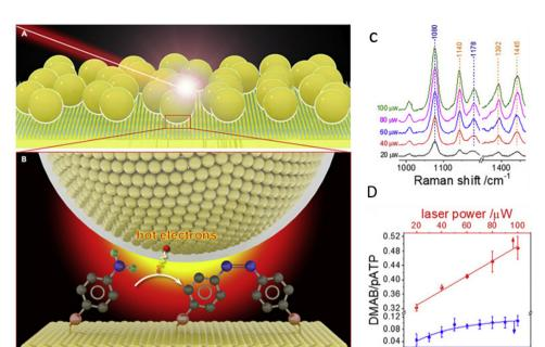
Fig. 18 (a) Scheme of in situ SERS study on the interfacial hot electron transfer in the photocatalytic conversion of p-aminothiophenol (p-ATP) to dimercaptoazobenzene (DMAB). (b) SERS spectra of the conversion of p-ATP catalyzed by Au NPs at different laser power excitations. (c) The relative intensity of DMAB to p-ATP bands with different incident laser powers. The figure is adapted from ref. 582 with permission from Springer, Copyright 2020.
