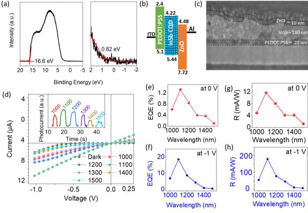
Fig. 3 (a) UPS spectra of sulfide-capped InSb CQDs with high- and low-binding energy cutoff regions. (b) Energy band diagram of the QPD under nobias condition. (c) Typical cross-sectional SEM image of the QPD stack. (d) I-V characteristics of the QPD in a linear form under different SWIR wavelengths of light; the inset shows the photoresponse of the QPD under different wavelengths of SWIR light. (e) and (f) EQE of the QPD and (g) and (h) responsivity of the QPD at 0 and -1 V, respectively.
