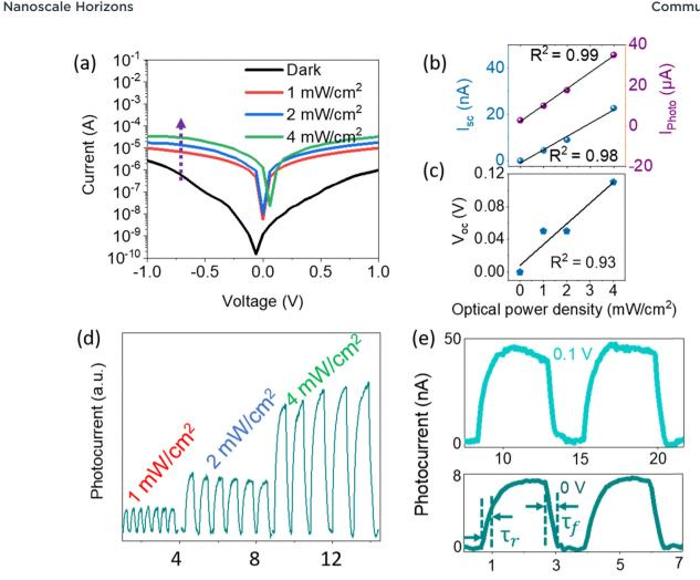
Fig. 4 (a) Logarithmic I-V characteristics of the QPD at 1100 nm with different optical light intensities. Optical illumination intensity-dependent (b) I<sub>SC</sub>,  $I_{\rm photo}$  (-1 V) and (c)  $V_{\rm oc}$  values (linear fit) of the QPD. (d) Photoresponse of the QPD at different light intensities of 1100 nm light. (e) Photoresponse of the QPD at 0 and 0.1 V.
