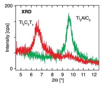
Fig. 7 XRD image of  $Ti_3AlC_2$  and  $Ti_3C_2T_x$ . The diffractogram shows the  $Ti_3AlC_2$  film at 9.65 and the  $Ti_3C_2T_x$  film at 6.60.<sup>45</sup>
