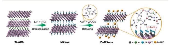
Fig. 3 Scheme for the Zr-MXene preparation.<sup>37</sup>
