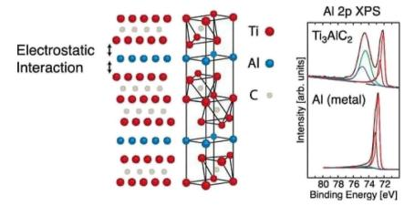
Fig. 6 X-ray photoelectron spectroscopy of Ti<sub>3</sub>AlC<sub>2</sub>. 45
