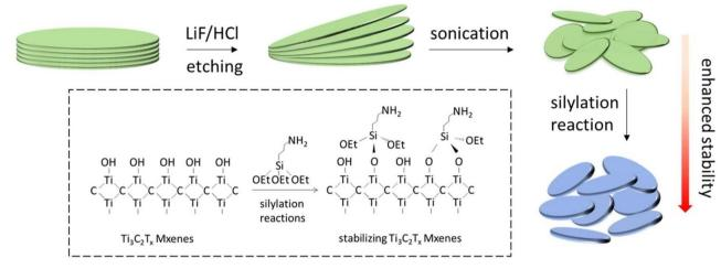
Selective etching and sonication of MXenes with LiF/HCl (copyright 2019 Elsevier)
