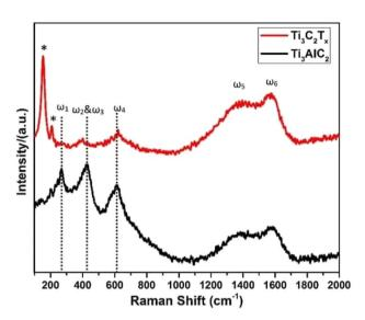
Fig. 5 The Raman spectra exhibit distinctive features for both  ${\rm Ti}_3{\rm AlC}_2$  MAX powder and  ${\rm Ti}_3{\rm C}_2{\rm T}_x$  MXene. Peaks labeled with "\*" specifically correspond to the out-of-plane vibrations of titanium (Ti) and carbon (C) atoms in the structure.
