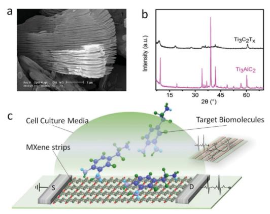
Fig. 17 Characterization of bulk MXenes. (a) SEM image of the multilayer structured MXene. (b) XRD patterns of the transition from Ti<sub>3</sub>AlC<sub>2</sub> to Ti<sub>3</sub>C<sub>2</sub>T<sub>x</sub>. (c) Schematic of a biosensing device based on MXene field effect transistors (copyright 2016 John Wiley and Sons).<sup>151</sup>
