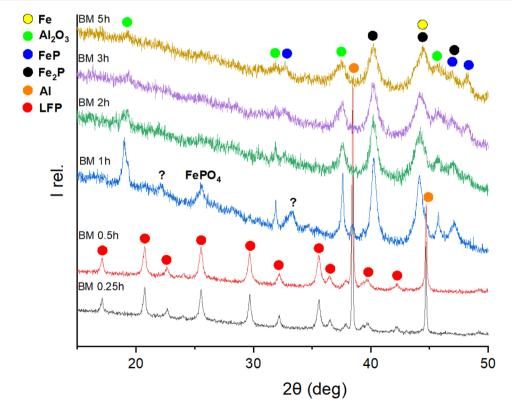
Fig. 2 XRD patterns of a 1:3 molar mixture of LFP and Al measured after different ball-milling times. The most intense Bragg-reflections are assigned to different phases for analysis. The reflections labeled with a question mark cannot be identified because the intensities are too low for a reasonable assignment to a matching phase. 2–3 h are necessary to finish the reaction.
