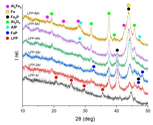
Fig. 5 XRD patterns of various molar mixtures of LFP and Al measured after 3 h of ball-milling. The most intense Bragg-reflections are assigned to different phases for analysis.  $X \approx 5.6$  for  $Al_xFe_2$ , identified by lattice parameters.
