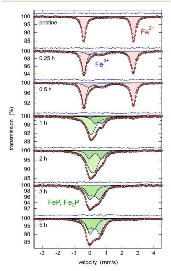
Fig. 3 Mössbauer spectra of pristine LFP and LFP ball-milled with Al metal foil for 0.25 h to 5 h (1:3 molar ratio of LFP to Al). The experimental data points are shown as white spheres, the overall fit as red line, the difference as blue line, and the subspectra are shown as red, blue, and green singlets/doublets
