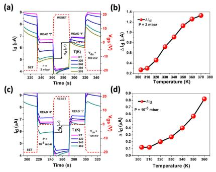
Fig. 5 (a) and (b) SET/READ/RESET/READ cycles and memory window versus temperature under 2 mbar pressure. (c) and (d) SET/READ/RESET/READ cycles and memory window *versus* temperatures under  $10^{-5}$  mbar pressure. Lines in (b) and (d) are guide to the eye
