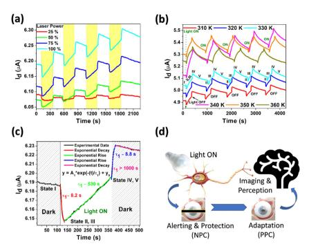
Fig. 6 (a) Transient photocurrent at different laser powers at 310 K,  $V_{ds} = 10$  mV. (b) Transient photocurrent at different temperatures with a maximum laser power, at  $V_{ds}$  = 100 mV. In both cases, the maximum laser power was 110 mW,  $10^{-5}$  mbar pressure, and  $V_{qs}$  = 0 V. (c) Current decay/rise and exponential fit at 310 K,  $10^{-5}$  mbar pressure. (d) Corresponding illustration of the obtained NPC and PPC for neuromorphic vision sensors.
