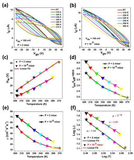
Fig. 4 (a) and (b) Transfer characteristics, (c) hysteresis width, (d) on/off current ratio, (e) and (f) mobility at different temperatures of the BP device under 2 mbar and  $10^{-5}$  mbar pressures. Lines in (d) and (e) are guide to the eye.
