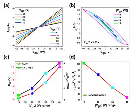
Fig. 2 (a) Output, (b) transfer characteristics, (c) hysteresis width and on/off current ratio, and (d) calculated mobility as a function of the gate voltage at RT and 2 mbar pressure. Lines in (c) and (d) are guide to the eye.
