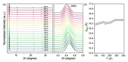
Fig. 7 (a) XRD patterns as a function of the temperature from 100 to 295 K for the (HA)<sub>2</sub>Snl<sub>4</sub>-based perovskite film and the XRD peak of the (002) facet; (b) the interlayer distance as a function of the temperature for the peak (002).
