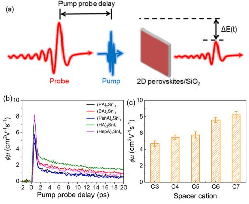
Fig. 4 (a) Photoconductivity dynamics by optical pump-THz probe (OPTP) spectroscopy. (b) Comparison of the mobility and free-carrier generation quantum efficiency  $(\phi_{\mu})$  for the five perovskites. (c) Charge carrier mobility (peak values in a) as a function of the chain length of the spacer cation.
