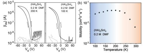
Fig. 6 Low temperature transfer characteristics of the (HA)<sub>2</sub>Snl<sub>4</sub>-based FET device at (a) 200 and 100 K. (b) Corresponding temperature-dependent field-effect mobility from 100 K to 295 K.
