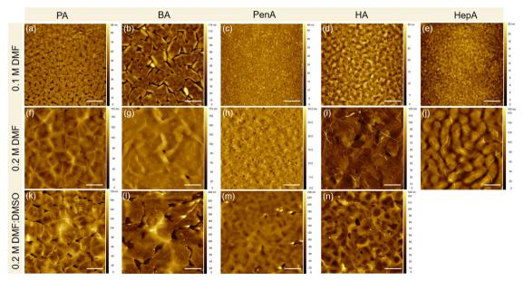
Fig. 2 AFM height images of 2D tin halide perovskite films with different spacers PA, BA, PenA, HexA, and HepA obtained under the processing conditions of (a)-(e) 0.1 M, DMF; (f)-(j) 0.2 M, DMF; (k)-(n) 0.2 M, DMF:DMSO, respectively. Scale bar: 10 µm.
