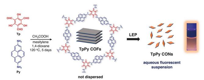
Fig. 2 Schematic diagram of the preparation of TpPy CONs by solvothermal condensation and liquid exfoliation process (fluorescent photograph of a 0.5 mg mL<sup>-1</sup> TpPy CON dispersion taken under 365 nm UV light). Adapted with permission from ref.79.
