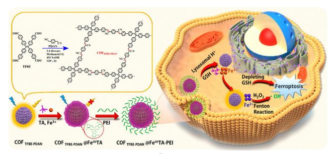
Fig. 3 Schematic illustration of the preparation of COF TFBE-PDAN@Fe<sup>III</sup>TA-PEI for luminescence imaging and ferroptosis in target tumor cells. Adapted with permission from ref. 80. Copyright 2022, American Chemical Society.
