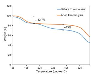
Fig. 6 TGA plots of monoUiO-66-NH<sub>2</sub>-30%-B (blue) and monoUiO-66-NH2-30%-A (orange).
