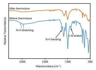
Fig. 3 FT-IR spectra of mono UiO-66-NH<sub>2</sub>-30%-B (blue) and mono UiO-66-NH<sub>2</sub>-30%-A (orange).
