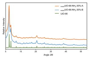
Fig. 1 Experimental PXRD patterns of mono UiO-66-NH<sub>2</sub>-30%-B and mono-UiO-66-NH<sub>2</sub>-30%-A and the simulated pattern for UiO-66.
