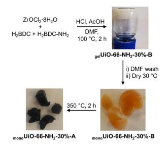
Scheme 1 Synthesis of  $_{\rm mono}$ UiO-66-NH $_2$ -30%-B (orange) and  $_{\rm mono}$ UiO-66-NH $_2$ -30%-A (black) from  $_{\rm gel}$ UiO-66-NH $_2$ -30%-B. H $_2$ BDC-NH $_2$  used was 30% by weight with respect to H $_2$ BDC.
