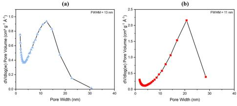
Fig. 5 The BJH pore distribution with FWHM analysis for (a) monoUiO-66-NH2-30%-B and (b) monoUiO-66-NH2-30%-A
