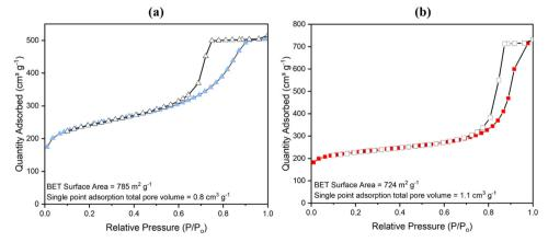
Fig. 4  $N_2$  gas adsorption isotherms measured at 77 K for (a)  $_{mono}$ UiO-66-NH $_2$ -30%-B (solid triangles represent adsorption, and open triangles denote desorption); (b)  $_{mono}$ UiO-66-NH $_2$ -30%-A (solid squares represent adsorption, and open squares denote desorption).
