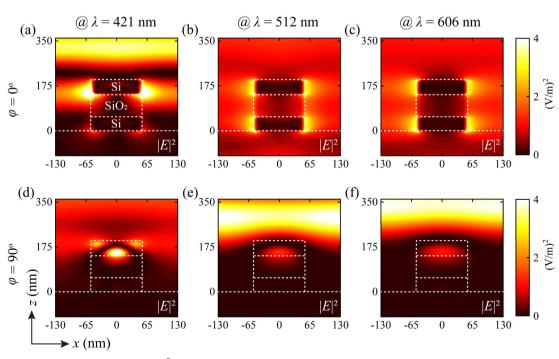
Fig. 3 The xz-view of the spatial electric field ( $|E|^2$ ) distributions at the wavelengths of 421, 512, and 606 nm for (a)–(c)  $\varphi = 0^\circ$  and (d)–(f)  $\varphi = 90^\circ$ . The white dotted lines denote the proposed dielectric metasurface structure.
