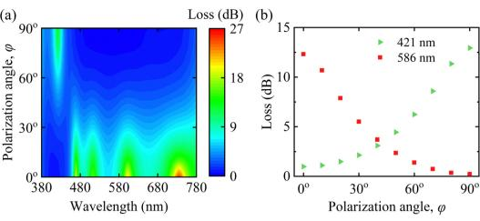
Fig. 10 (a) Loss profile due to change of  $\varphi$  from 0° to 90° at operating wavelengths from 380 nm to 780 nm of our proposed dielectric grating metasurface. (b) Loss at the wavelengths of 421 and 586 nm for varying  $\varphi$ . Here, we considered the resonance wavelengths at  $\varphi$  values of 0° and 90°.
