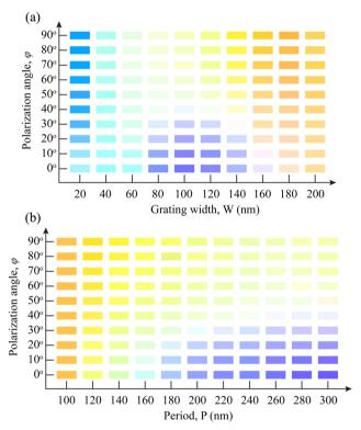
Fig. 7 (a) A color palette of our proposed structure for varying W and  $\varphi$ . We adopted a range of W from 20 to 200 nm. Here, we rotated the  $\varphi$  from 0° to 90°. (b) A color palette of our proposed dielectric metasurface structure for varying P and  $\varphi$ . We adopted a range of P from 100 to 300 nm. Here, we rotated the  $\varphi$  from 0° to 90°.
