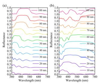
Fig. 4 Reflectance spectra of the dielectric metasurface structure for different  $t_{Si}$  values at (a)  $\varphi = 0^{\circ}$  and (b)  $\varphi = 90^{\circ}$ . Other structural parameters were kept constant
