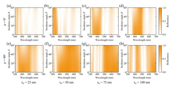
Fig. 9 Reflectance spectra for different thicknesses of Si layer of our proposed grating dielectric metasurface with varying  $\theta$  values for the  $\varphi$  of (a) – (d) 0° and (e)–(h) 90°. In this case,  $t_{Si}$  increases from 25 to 100 nm, and the  $\theta$  increases from 0° to 60°.
