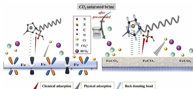
Fig. 20 Protective mechanism of DMIMHS towards the corrosion inhibition of Fe and FeCO<sub>3</sub> surface. [Reprinted with permission from ref. 119, ©2022 Elsevier.]
