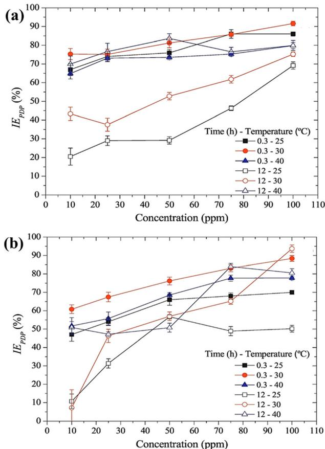
Fig. 7 After evaluating API-X52 steel as a working electrode in the presence of 1 M HCl solution, the inhibition efficiency of (a) TMA and (b) TTA as functions of the immersion duration and temperature [reprinted with permission from ref. 90, ©2018 Elsevier].
