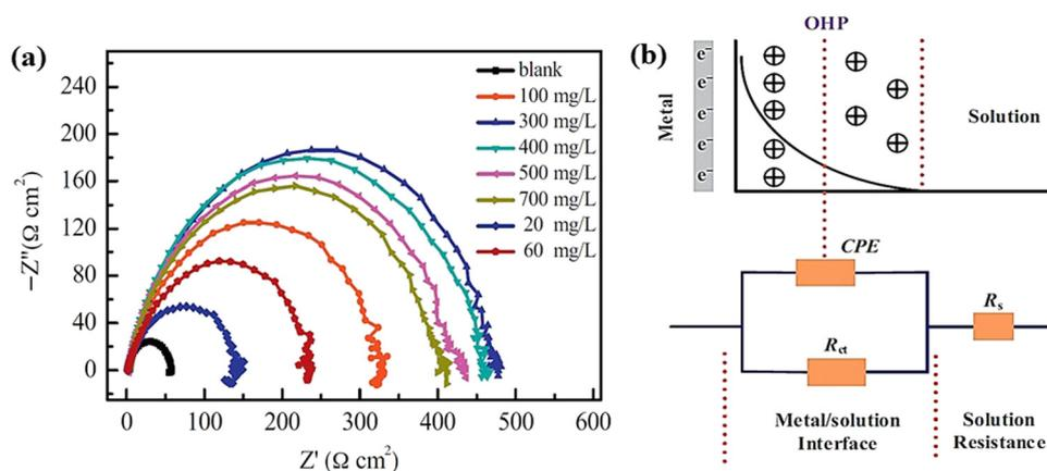
Fig. 6 (a) Nyquist plot for the carbon steel working electrode in the presence of 0.1 M H<sub>2</sub>SO<sub>4</sub> solution without and with different concentrations of BKC, (b) potential distribution diagram at the interface between the metal and the electrolytic solution (above) and analogous circuit used to fit the Nyquist plot (below) [reprinted with permission from ref. 95, ©2015 Elsevier].
