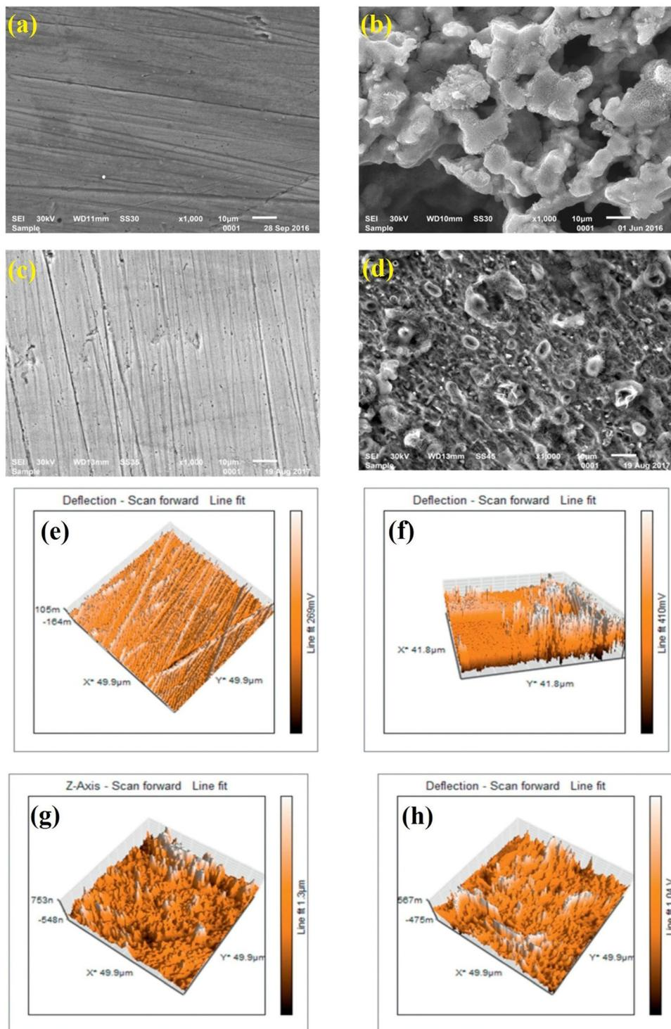
Fig. 13 SEM (a–d) and AFM (e–h) images of (a and e) the polished mild steel, (b and f) after immersion within 0.5 M  $\text{H}_2\text{SO}_4$  without IL, (c and g) with  $10^{-2}$  M [FBMIm]Br, and (d and h) with  $10^{-5}$  M [FBMIm]Br. [Reprinted with permission from ref. 126, ©2019 Elsevier.]
