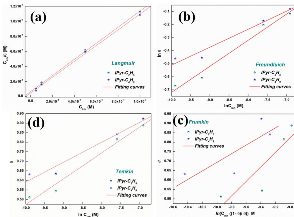
Fig. 10 (a) Langmuir, (b) Freundlich, (c) Frumkin and (d) Temkin isotherm models for understanding the adsorption mechanism of IPyr-C<sub>2</sub>H<sub>5</sub> and IPyr-C<sub>4</sub>H<sub>9</sub> on mild steel surface in the presence of 1 M HCl at 298 K. [Reprinted with permission from ref. 103, ©2020 Elsevier.]
