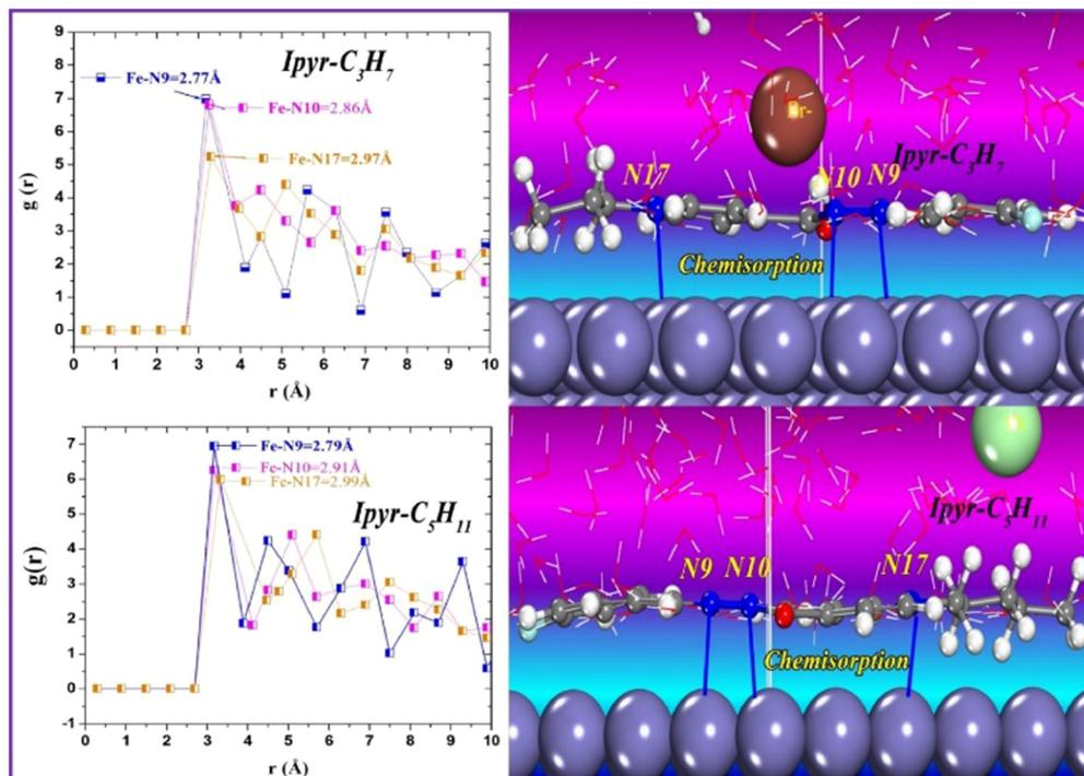
Fig. 18 RDF analysis of adsorbed Ipyr-C3H7 and Ipyr-C5H11 on Fe(110) surface in a simulated acid medium at 298 K temperature obtained from MD simulation. [Reprinted with permission from ref. 104, ©2021 Elsevier.]
