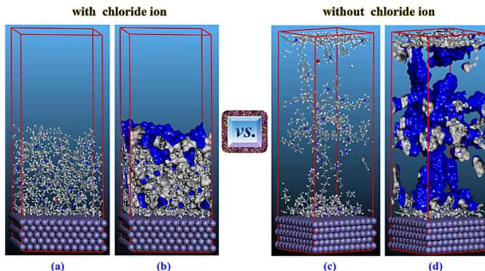
Fig. 22 (a) and (c) Equilibrium configuration and (b) and (d) free volume distribution of the inhibitor film of BKC cations with and without chloride ions. [Reprinted with permission from ref. 95, ©2015 Elsevier.]
