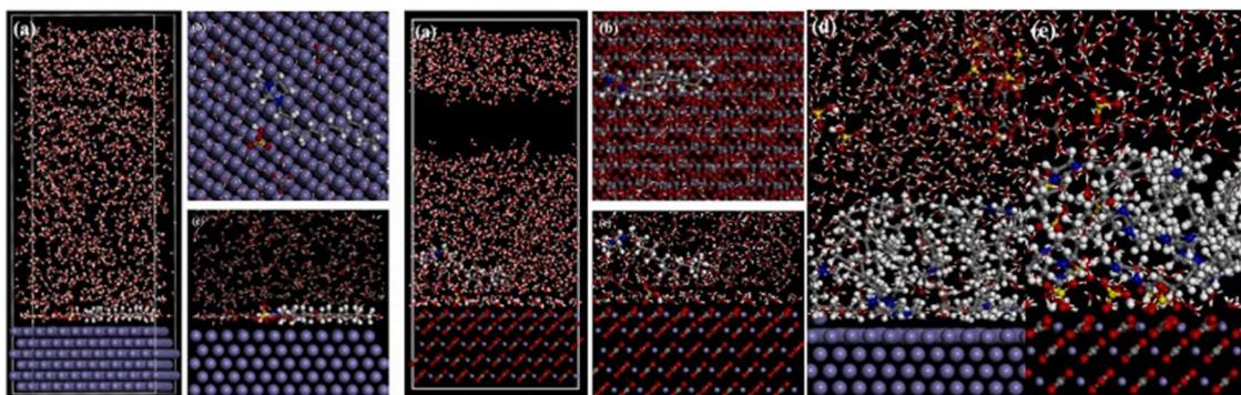
Fig. 19 Optimized adsorption configuration of the adsorption of one DMIMHS on Fe(110) (first column) and FeCO<sub>3</sub>(104) (middle two columns): (a) overall view, (b) top view and (c) side view; optimized adsorption configuration of nine DMIMHS on (d) Fe(110) and (e) FeCO<sub>3</sub>(104). [Reprinted with permission from ref. 119, ©2022 Elsevier.]
