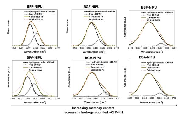
Fig. 1 Deconvoluted hydroxyl region in the ATR-FTIR spectra of the NIPUs. The -OH/-NH absorption bands were fit using two Gaussian distributions: one for hydrogen-bonded -OH/-NH groups and another for free -OH/-NH groups.
