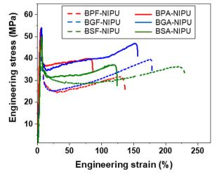
Fig. 2 Representative tensile engineering stress vs. engineering strain curves for NIPUs acquired from uniaxial tensile testing using a load cell of 100 N and a strain rate of 10% min<sup>-1</sup> at  $\sim$ 20 °C.
