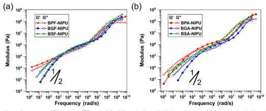
Fig. 5 Frequency-dependent storage (G') and loss (G") moduli for (a) unsubstituted bridging carbon- and (b) dimethyl-substituted bridging carbonbased NIPUs. The master curves were constructed using time-temperature superposition and reported at 150 °C. Lines indicate typical power-law scalings of G' (slope of 2) and G'' (slope of 1)
