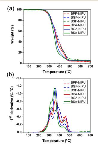
Fig. 4 (a) TGA thermograms of NIPUs in  $N_2$  atmosphere; sample weight (%) as a function of temperature with a heating rate of 10 °C min<sup>-1</sup>, and (b) the first derivative of the weight remaining (%/°C) as a function of temperature for all NIPUs.
