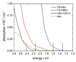
Fig. 13 Onset of the unpolarized theoretical absorption spectrum (TB-mBJ, YS-PBE0, TB-mBH+U (4.08) functionals) in comparison with the experimental (exp.) data. The arrows mark the corresponding band gaps.
