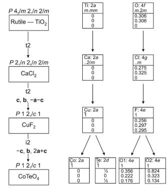
Fig. 3 Bärnighausen tree showing the symmetry relationship between the rutile aristotype and the CoTeO<sub>4</sub> hettotype.
