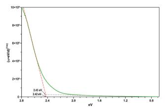
Fig. 14 Direct bandgap Tauc plot derived from the unpolarized transmission spectrum of CoTeO<sub>4</sub> using a crystal plate with a thickness of  $\sim$ 5  $\mu m$ .
