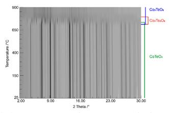
Fig. 5 Temperature-dependent SPXRD in situ study of CoTeO<sub>4</sub> using a wavelength of 0.4087 Å. The existence range of present phases is indicated on the right.
