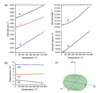
(a) Evolution of unit-cell parameters with temperature; (b) depen-Fia. 7 dence of eigenvalues of the thermal expansion; (c) three-dimensional surface of the thermal expansion tensor for CoTeO<sub>4</sub> (500 °C data).
