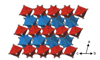
Fig. 4 Projection of the dirutile-type crystal structure of CoTeO<sub>4</sub> along [011]. [CoO<sub>6</sub>] octahedra are given in blue, [TeO<sub>6</sub>] octahedra in red. Displacement ellipsoids are drawn at the 90% probability level.
