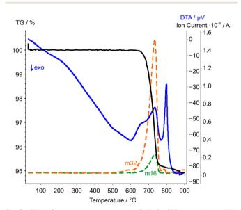
Fig. 6 STA-MS measurement curves of CoTeO<sub>4</sub> (TG curve black, DTA curve blue). Only the mass signals (dashed lines) with significant intensities with respect to the ion current are displayed.
