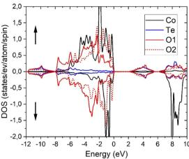
Fig. 11 Spin-polarized partial DOS of CoTeO<sub>4</sub> in the TB-mBJ+U (4.08 eV) approximation.
