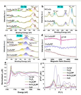
Fig. 2 (a)–(c) High-resolution Co 2p, Ni 2p and S 2p XPS spectra of the relevant samples. (d) EPR spectra of  $Co_9S_8$ ,  $Ni-Co_9S_8$ , and  $Co_9S_8/BP$ , respectively. (e) XANES and (f) EXAFS spectra of Co, CoO, Co<sub>9</sub>S<sub>8</sub>, Co<sub>9</sub>S<sub>8</sub>/ BP and Ni-Co<sub>9</sub>S<sub>8</sub>/BP, respectively
