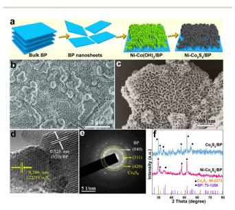
Fig. 1 (a) Synthesis diagram of the Ni-Co<sub>9</sub>S<sub>8</sub>/BP heterostructure. SEM images of (b) Ni-Co(OH)<sub>2</sub>/BP and (c) Ni-Co<sub>9</sub>S<sub>8</sub>/BP. (d) HRTEM and (e) SAED images of Ni-Co<sub>9</sub>S<sub>8</sub>/BP. (f) XRD patterns of Co<sub>9</sub>S<sub>8</sub>/BP and Ni-Co<sub>9</sub>S<sub>8</sub>/ BP, respectively.
