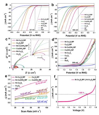
Fig. 3 HER polarization curves of relevant samples in (a) 0.5 M H<sub>2</sub>SO<sub>4</sub> and (b) 1 M KOH, respectively. (c) EIS spectra (the inset shows the enlarged area of the pink dotted line). (d) OER polarization curves of relevant samples in 1 M KOH. (e) Current-potential curves with different scan rates in 1 M KOH. (f) Polarization curves of overall water splitting based on the Ni-Co<sub>9</sub>S<sub>8</sub>/ BP||Ni-Co<sub>9</sub>S<sub>8</sub>/BP couple.
