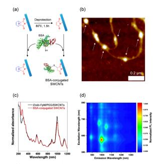
Fig. 5 (a) Schematic of BSA modification experiments on endo-FpM/ PEG/SWCNTs. (b) Representative AFM image of BSA-conjugated SWCNTs. (c) Normalized absorption spectra of endo-FpM/PEG/SWCNTs before (black) and after (red) the BSA conjugation. (d) PL contour plot of endo-FpM/PEG/SWCNTs after BSA conjugation.
