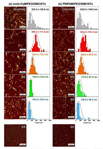
Fig. 3 AFM images and length distribution of unsorted, fr1, fr2, fr3, fr4, and fr5 of (a) endo-FpM/PEG/SWCNTs and (b) PNIPAM/PEG/SWCNTs. Displayed values are mean length  $\pm$  standard deviation for N=50.
