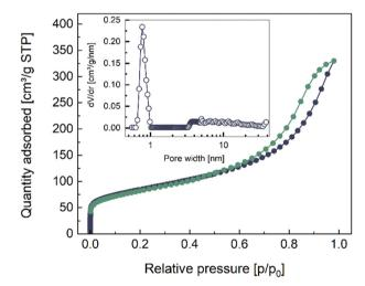
Fig. 2 N<sub>2</sub> adsorption (black) and desorption (green) isotherms of the Ti<sub>9</sub>O<sub>17</sub> nanowires synthesized in saturated KOH via electrochemical erosion. The inset shows the pore size distribution with a strong peak around  $\sim 0.8$  nm.
