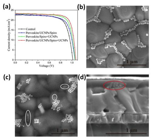
Fig. 15 (a) J-V characteristics of several types of PSCs. Top-view SEM images of (b) perovskite/UCNP film and (c) perovskite/UCNP/spiro + UCNP film. (d) Cross-sectional SEM images of the PSC with the structure of ITO/SnO<sub>2</sub>/perovskite/UCNPs/spiro + UCNPs/Au. Reprinted with permission from the American Chemical Society.93
