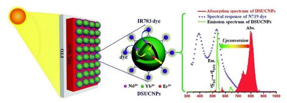
Fig. 6 Broadband near-infrared sunlight harvesting and spectral conversion into the visible range to activate the N719 dye for the improvement of a DSSC device. Reprinted with permission from Elsevier.<sup>84</sup>
