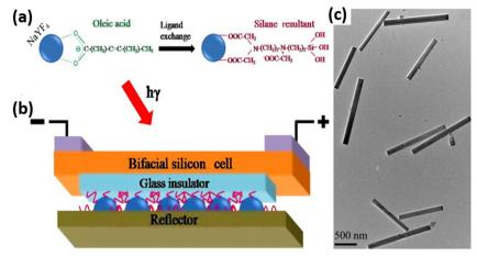
Fig. 19 (a) Ligand exchange of NaYF<sub>4</sub>:Er nanocrystals. (b) A schematic of upconversion film application in silicon solar cells. (c) TEM image of NaYF<sub>4</sub>:Er nanocrystals dispersed in methanol after ligand exchange. Reprinted with permission from Elsevier.<sup>76</sup>
