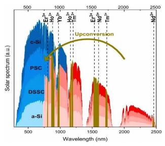
Fig. 1 Parts of the solar spectra of different solar cell types, utilized (in blue) and lost (in red), and the absorption ranges (in brown) of the upconverting Ln<sup>3+</sup> ions.<sup>11</sup>
