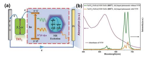
Fig. 10 (a) Energy diagram illustrating the NIR light-harvesting by the N719 dye through the UC process, the charge injection into  $TiO_2$  and the transport of photoelectrons to the electrode surface. (b) The absorption spectra of the N719 dye and the UC emission spectra of  $TiO_2$  photoanodes with NaYF<sub>4</sub>:Yb<sup>3+</sup>/Er<sup>3+</sup>@YOF:Yb<sup>3+</sup>/Er<sup>3+</sup> (600 °C, air) before and after immersion in N719 dye. Reprinted with permission from Wiley.<sup>88</sup>
