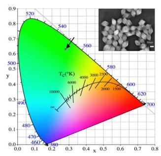
**Fig. 12** The CIE chromaticity diagram of Li(Gd,Y)F<sub>4</sub>:Yb,Er (inset: the TEM image of Y<sup>3+</sup>-doped LiGdF<sub>4</sub>:Yb<sup>3+</sup>,Er<sup>3+</sup> upconversion nanocrystals). Reprinted with permission from Elsevier.<sup>68</sup>
