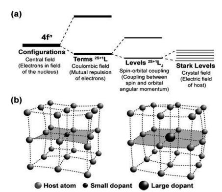
Fig. 4 (a) A simplified representation of the effect of the coulombic field, spin-orbit coupling, and crystal-field interaction on the [Xe]4f<sup>n</sup> configuration. (b) Crystal lattice contraction (left) and expansion (right) as a result of the substitution of a host atom with dopants of varied sizes. Reprinted with permission from Wiley.<sup>53</sup>
