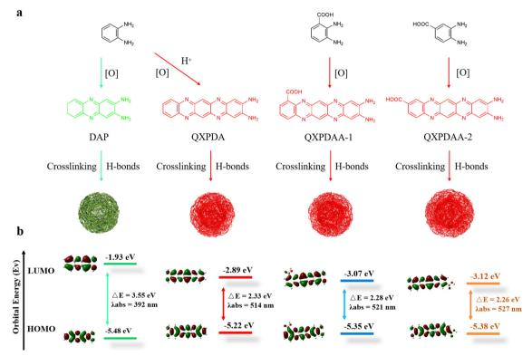
Fig. 4 (a) Schematic diagram of the preparation of the proposed DAP, QXPDA, QXPDAA-1 and QXPDAA-2. (b) Theoretical calculations of DAP, QXPDA, QXPDAA-1 and QXPDAA-2 at the (TD-DFT) B3LYP/6-31G (d, p) level. HOMO: the highest occupied molecular orbital, LUMO: the lowest unoccupied molecular orbital.
