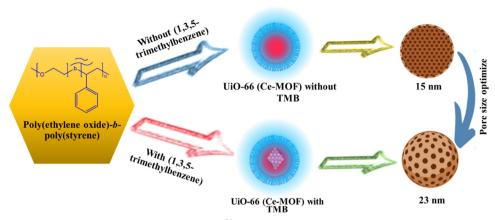
Fig. 2 Porosity of Ce-MOFs optimized using 1,3,5-trimethylbenzene.<sup>52</sup>
