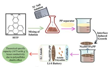
Fig. 6 The application of MOFs in lithium sulfur batteries. 116
