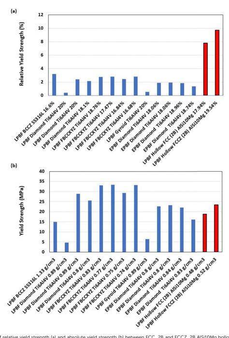
Fig. 8 Comparison of relative yield strength (a) and absolute yield strength (b) between FCC\_2B and FCCZ\_2B AlSi10Mg hollow-strut lattices and Ti-6Al-4V and SS316L solid-strut lattices of similar relative density (17-20%). 53,54,78-82 The name of each data point on the X-axis denotes "unit cell topology, material, relative or absolute density". Error bars were not included as the standard deviation between samples was negligible
