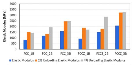
Fig. 7 Normal elastic moduli (blue) and unloading elastic moduli (yellow and grey) of AlSi10Mg FCC and FCCZ HSLs. (1B) single border scan (ΔD = 240  $\mu$ m). 2B: double border scans ( $\Delta D = 390 \mu$ m). 3B: triple border scans ( $\Delta D = 540 \mu$ m). Error bars were not included as the standard deviation between samples was negligible
