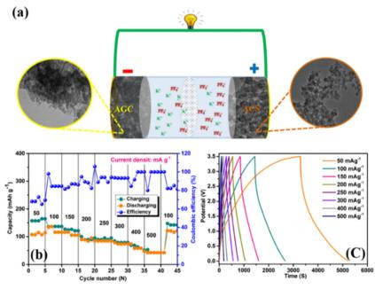
Fig. 8 Electrochemical performance of the AGC//ACS K-ion capacitor: (a) schematic illustration of the fabrication of the KIC full cell, (b) rate capability at current densities from 50 to 500 mA g<sup>-1</sup>, and (c) GCD curves recorded at different current densities.
