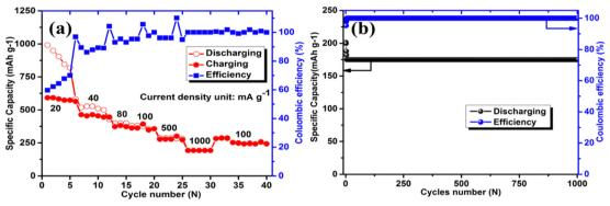
Fig. 7 (a) Rate capability at current densities from 20 to 1000 mA g<sup>-1</sup> and (b) long-term cycling performance at 1000 mA g<sup>-1</sup> of AGC.
