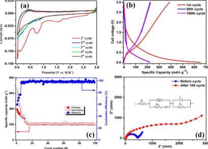
Fig. 6 (a) Cyclic voltammogram of the synthesized AGC anode cycled between 0.1 and 3.0 V vs. K $^+$ /K with the scan rate of 0.05 mV s $^{-1}$ . (b) Discharge-charge profiles of the AGC anode at 100 mA g $^{-1}$ . (c) Cycling stability and coulombic efficiency of the AGC anode at the current density of 100 mA g $^{-1}$ . (d) EIS spectra of the as-fabricated AGC anode (blue color) and the cell under the influence of 100 mA g $^{-1}$  after 100 cycles (red color) and the fitted equivalent circuit.
