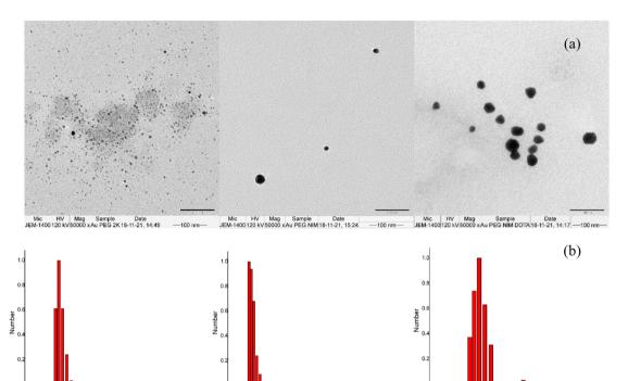
Fig. 3 (a) TEM images of AuNP-PEG-2K-NH2, AuNP-PEG-2K-(2-NIM) and AuNP-PEG-2K-(2-NIM)(DOTA) [left to right]. (b) Size distribution data of AuNP-PEG-2K-NH<sub>2</sub>, AuNP-PEG-2K-(2-NIM) and AuNP-PEG-2K-(2-NIM)(DOTA) [left to right].
