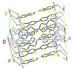
Fig. 3 Crystal structure of  $\alpha$ -ET<sub>2</sub>I<sub>3</sub>. The blue, yellow, open, and green spheres indicate C, S, H, and I atoms, respectively. The broken lines indicate the (C-)H···I and (C-)H···S contacts that are shorter than the van der Waals distances (3.35 and 3.05 Å, respectively). At 296 K, a, b, and c = 9.17584(13), 10.79078(17), and 17.4193(3) Å, and  $\alpha$ ,  $\beta$ , and  $\gamma$  = 96.9633(13), 97.9521(13), and 90.8572(12)°, respectively.
