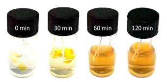
Fig. 9 Degradation process of VTCO-IPDI at different times in a 1 M HCl H<sub>2</sub>O/HFP (1/9, v/v) solution.
