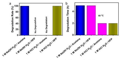
Fig. 10 (a) Degradation rate of VTCO-IPDI in 1 M HCl or 1 M NaOH solutions (H<sub>2</sub>O/solvent = 1/9, v/v). (b) Degradation time in 1 M HCl or 1 M NaOH solutions (H<sub>2</sub>O/solvent = 1/9, v/v) at 60 °C.
