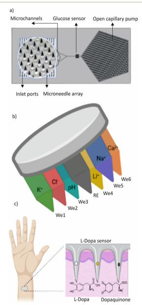
Fig. 6 a) Conceptual illustration of a microfluidic chip with porous microneedles (MNs) to collect ISF. b) Graphical representation of the MIMN patch. c) Microneedle sensing platform for continuous and minimally invasive monitoring of levodopa.
