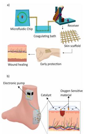
Fig. 8 a) Illustration of microfluidic spinning and collection of dualcargo-loaded microfibers. These biocompatible fibres are used for quick haemostasis and wound healing. b) Schematic representation of the oxygen sensing and delivery patch for foot ulcers and crosssectional view of the smart patch and wound area.
