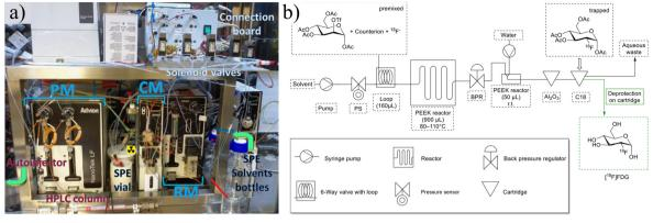
Fig. 4 a) The Advion Nanotek provides an automated method to produce radiotracers but requires significant and complicated setup. Reprinted from ref. 48 with permission from Elsevier. b) Schematic of FOMSy system with incorporated reactors and external SPE cartridges. Used with permission of Springer Nature from ref. 81; permission conveyed through Copyright Clearance Center, Inc.
