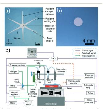
Fig. 10 a) The original passively-held droplet design used a star-like shape to create transport channels for reagents to collect into a single reaction site.  $^{113}$  b) Later iterations eliminated the channels in favor of dispensing the various reagents directly onto the reactions site using c) an automated microdropping system. 116 Used with permission of Royal Society of Chemistry from ref. 113 and 116; permission conveyed through Copyright Clearance Center, Inc.
