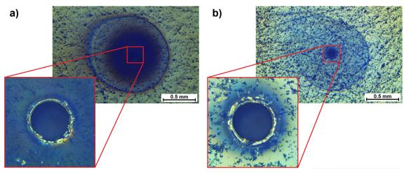
Fig. 1 (a) Optical microscope images of 90  $\mu$ m craters on NIST SRM 610 formed with 600 pulses of 13 J cm<sup>-2</sup> in nitrogen. A close-up framed in red is provided to represent the area visible during analysis. (b) Crater generated in helium using the same number of laser pulses as in (a).
