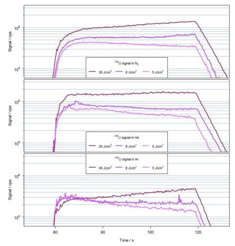
Fig. 4 Transient signal  $^{238}$ U<sup>+</sup> observed for 600 laser pulses at 10 Hz with a spot size of 90  $\mu$ m on NIST SRM 610 in helium (top), nitrogen (middle) and argon (bottom) with various fluences.
