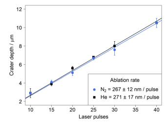
Fig. 7 Ablation rates determined by LSM for NIST SRM 610 in nitrogen (blue) and helium (black) using a fluence of 18 J cm $^{-2}$ . The error bars indicate the range of depths measured within an ablation crater (n=2).
