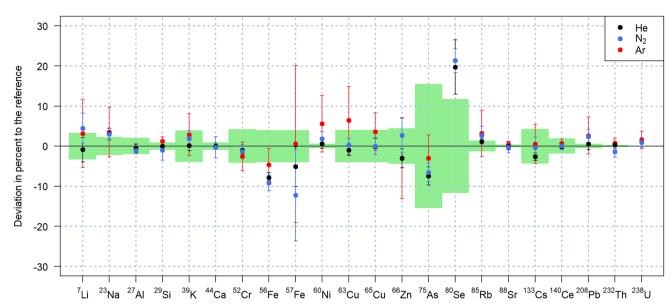
Fig. 3 Quantification of NIST SRM 612 using different carrier gases and NIST SRM 610 as calibration standard. <sup>40</sup>Ca was used as internal standard  $(^{4\bar{A}}$ Ca for measurements performed in argon) and a fluence of 19 J cm $^{-2}$  was applied. Error bars represent the standard deviations of 6 replicate analyses, while the standard deviations of the reference values are indicated by the light green areas.
