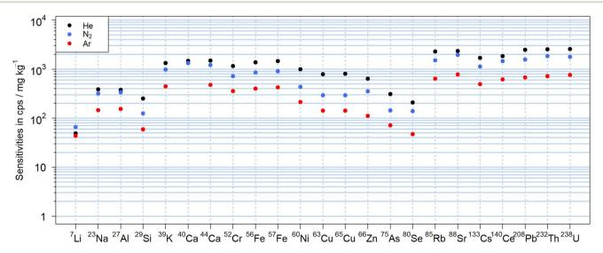
Fig. 2 Abundance normalized sensitivities obtained using helium (black), nitrogen (blue) or argon (red) as carrier gas using the average signal over 600 pulses of 90  $\mu$ m at 10 Hz and 19 J cm<sup>-2</sup> LA of NIST SRM 610.
