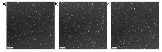
Fig. 13 Scanning transmission electron microscopy images of laser-generated aerosol formed in nitrogen (a), helium (b) and argon (c) in a two-volume cell. Scale bar is  $1 \mu m$ . Most agglomerates are found to be below the micrometer scale for all carrier gases and adopted filament structures of similar sizes
