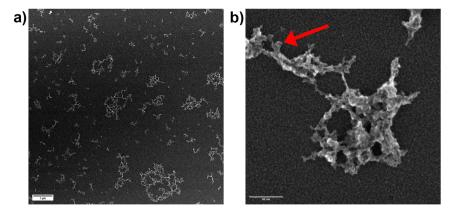
Fig. 11 (a) Secondary electron images of the laser-generated aerosol formed in helium visualized by scanning transmission electron microscopy with the scale bar size set at  $1 \mu m$ . (b) Higher magnification of a single agglomerate enabling the observation of the primary particles with the scale bar set at 50 nm and a red arrow was added to indicate a primary particle.
