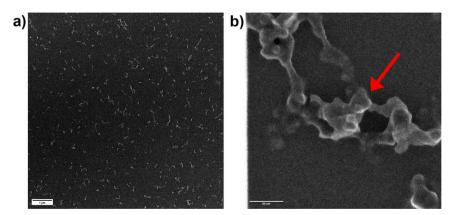
Fig. 10 (a) Secondary electron images of the laser-generated aerosol formed in argon visualized by scanning transmission electron microscopy with the scale bar size set at  $1 \mu m$ . (b) Higher magnification of a single agglomerate enabling with the scale bar set at 50 nm and a red arrow was added to indicate a preliminary particle.
