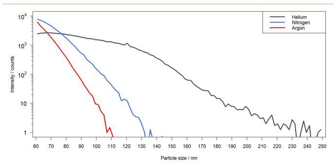
Fig. 8 Particle size distribution measured over 4 replicates for the laser-generated aerosol formed in helium (black), nitrogen (blue) and argon (red) by OPC.
