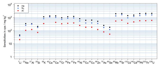
Fig. 12 Sensitivities obtained with 600 pulses of 90  $\mu$ m at 10 Hz and 18 J cm<sup>-2</sup> on NIST SRM 610 using a two-volume cell with the main volume flushed with helium (black), nitrogen (blue) or argon (red). The difference in sensitivities was similar to those observed with a cylindrical cell for the various carrier gases.
