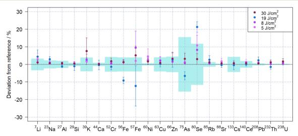
Fig. 6 Quantification of NIST SRM 612 using different fluences and NIST SRM 610 as calibration standard. <sup>40</sup>Ca was used as internal standard and nitrogen as carrier gas. Error bars represent the standard deviations of 4 replicate analysis, while the standard deviations of the reference values are indicated by the light blue areas.
