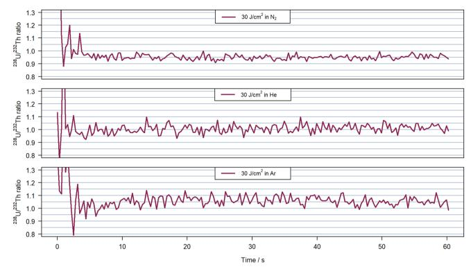
Fig. 5  $^{238}$ U<sup>+</sup>/ $^{232}$ Th<sup>+</sup> ratio measured for 30 J cm<sup>-2</sup> in nitrogen at 0.951(18) on average (top), helium at 1.01(3) (middle) and argon at 1.06(3) (bottom) with 600 pulses at 10 Hz on NIST SRM 610. The time window illustrates the 60 s of ablation without background nor washout time. The  $^{238}$ U<sup>+</sup> transient signal corresponding to the experiment presented here can be visualize in Fig. 4 at the corresponding fluence and carrier gas.
