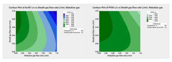
Fig. 3 Contour plots of blank-subtracted signal intensity of 5  $\mu$ g L<sup>-1</sup> Au (left) and Pt (right) from multivariate optimizations of sheath gas flow rate and nebulizer gas flow rate on the Varian 820MS using the 50-2 mm MC IR-heated at 110  $^{\circ}$ C and a 50  $\mu$ L min<sup>-1</sup> sample uptake rate.
