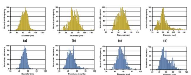
Fig. 6 Examples of normalized particle size distribution using NexION 2000 for 60 nm Au NPs (a–d) and 50 nm Pt NPs (e–h) measured by unheated cyclonic spray chamber (a and e); 25-2 mm MC IR-heated at 70 °C (b and f); 50-2 mm MC IR-heated at 110 °C (c and g); and 75-2 mm MC IR-heated at 120 °C (d and h).
