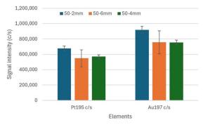
Fig. 4 Blank-subtracted signal intensity for 5  $\mu$ g L<sup>-1</sup> multielement solution with 110 °C IR-heated 50-2 mm, 50-4 mm and 50-6 mm MC spray chambers for Pt and Au with Varian 820MS.
