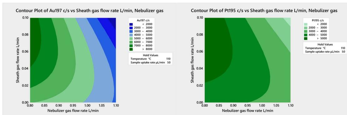
**Fig. 3** Contour plots of blank-subtracted signal intensity of 5  $\mu\text{g L}^{-1}$  Au (left) and Pt (right) from multivariate optimizations of sheath gas flow rate and nebulizer gas flow rate on the Varian 820MS using the 50-2 mm MC IR-heated at 110 °C and a 50  $\mu\text{L min}^{-1}$  sample uptake rate.
