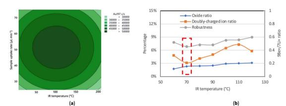
Fig. 2 Results of optimizations for 25-2 mm MC (a) Contour plot of blank-subtracted signal intensity for 5  $\mu$ g L<sup>-1</sup> Au vs. sample uptake rate and IR heating temperature; (b) oxide ratio, doubly charged ion ratio and robustness (Be+/Li+ signal ratio)<sup>27</sup> at different IR heating temperatures while other parameters were held constant. The optimum temperature is indicated by the dashed red box.
