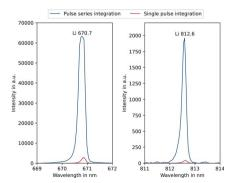
Fig. 2 Influence of the integration setting on the intensity of selected lithium emission lines (1 mg  $\rm L^{-1}$  Li) comparing measurement settings A (pulse series integration) and D (single pulse integration).
