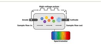
Fig. 1 By applying high-voltage pulses to the electrodes, a microplasma with an electron temperature of approx. 10 000 K is generated by a corona discharge at the cathode directly inside the liquid sample.
