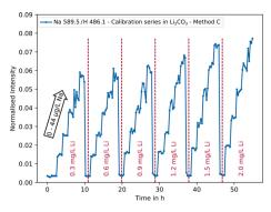
Fig. 6 Normalised intensity of the Na 589.5 nm emission line as a function of sodium (0–44  $\mu$ g L<sup>-1</sup>) and lithium concentrations (0.3–2.0 mg L<sup>-1</sup>) using parameter setting *C*.
