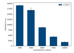
Fig. 4 Influence of the conductivity on the intensity of the Li 670.7 nm emission line (500  $\mu$ g L<sup>-1</sup> Li, n = 5).
