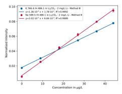
Fig. 5 Calibration curves of the Na 589.5 nm and K 766.4 nm emission lines in lithium carbonate solution containing 2 mg L<sup>-1</sup> Li using parameter setting B (n = 5).
