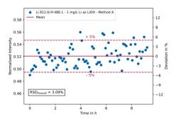
Fig. 7 Long-term (>9 hours) stability measurement of a lithium hydroxide solution containing 1 mg  $\rm L^{-1}$  Li using parameter setting A. The normalised intensity of the Li 812.6 nm emission line is plotted against time. The secondary y-axis shows the relative deviation in % around the mean value.
