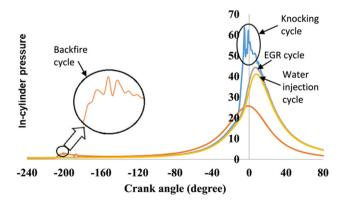
**Fig. 8** Control of combustion anomalies with EGR and water injection. Re-drawn from ref. 78.
