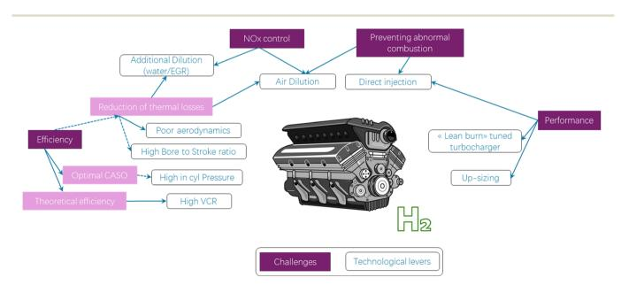
Fig. 16 Technological and control measures for addressing various challenges associated with hydrogen engines. Re-drawn from ref. 61.
