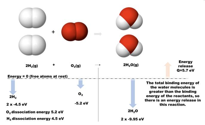
Fig. 4 Chemical process of hydrogen combustion. Re-drawn from ref. 59.
