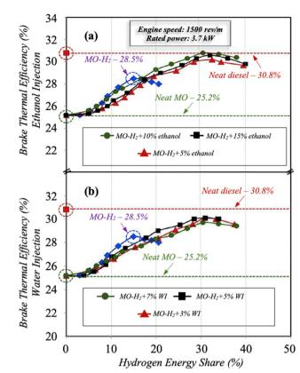
Fig. 6 Variation of BTE with different (a) ethanol injection amounts (b) water injection amounts. MO: *Madhuca longifolia* oil. Re-drawn from ref. 75.
