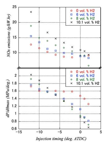
Fig. 11 Variations of  $NO_x$  and  $dP/d\theta_{max}$  with diesel fuel injection timing for different hydrogen fractions. Re-drawn from ref. 110 and 111.
