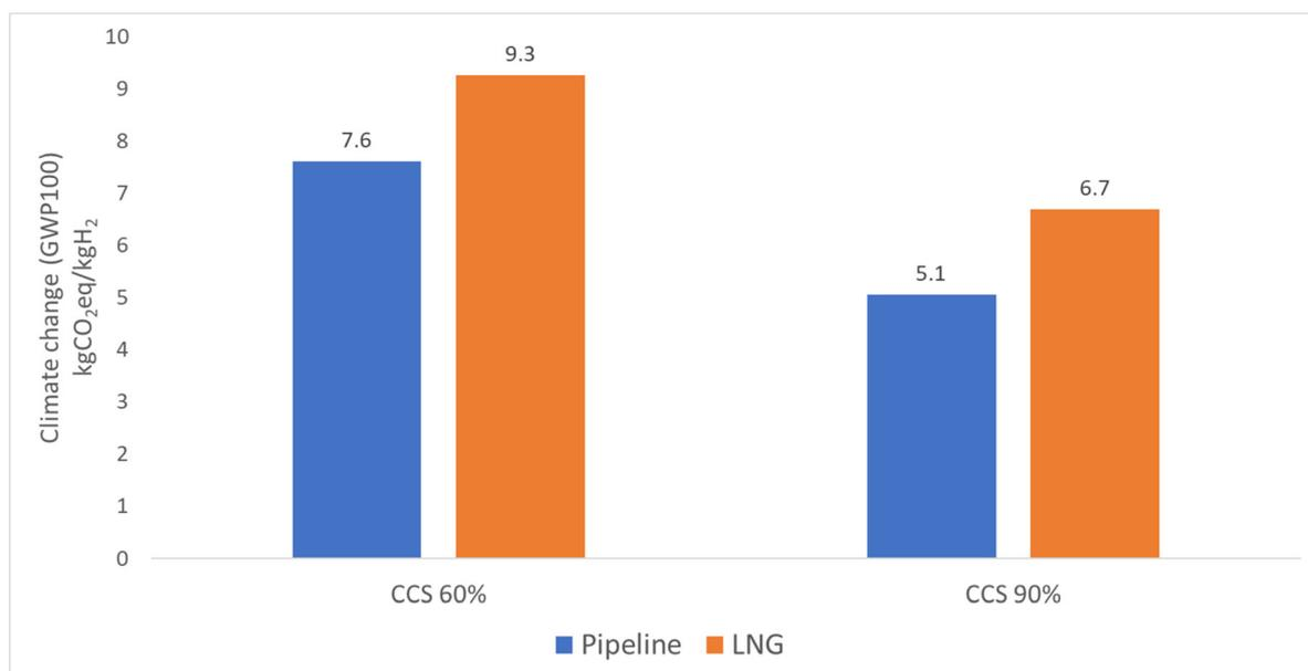
Fig. 10 Blue hydrogen CO<sub>2</sub> capture rate of 60% vs. 90%.
