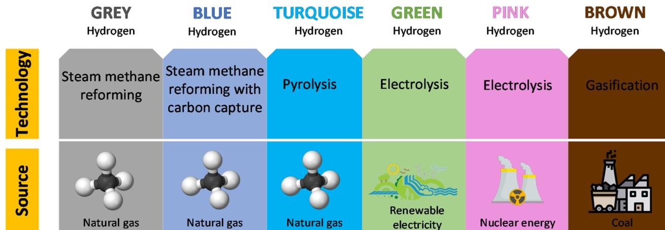
Fig. 1 The spectral colors of hydrogen based on the production method (modified from Renewable Energy Agency, 2020).<sup>9</sup>
