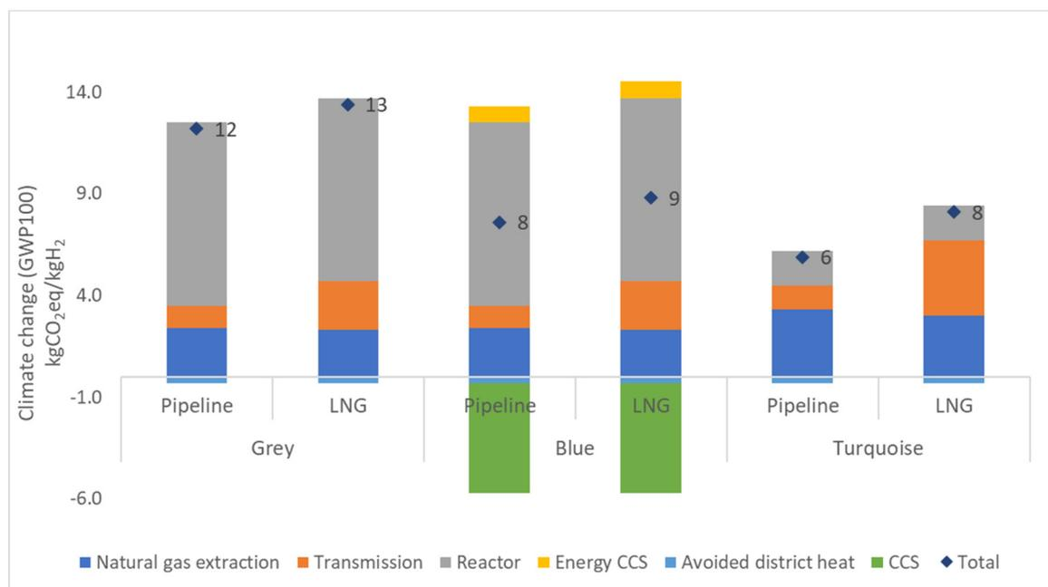
Fig. 6 LCIA results of examined hydrogen production technologies (Climate change, GWP 100).
