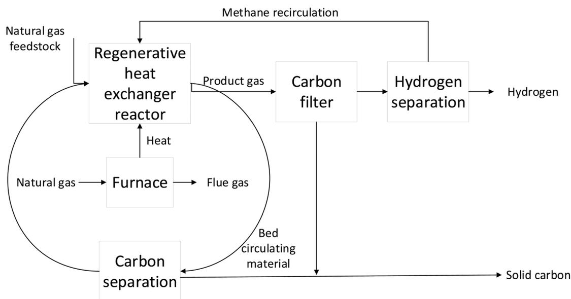
Fig. 4 Turquoise hydrogen (TDM) production (modified from Keipi et al., 2018).<sup>25</sup>
