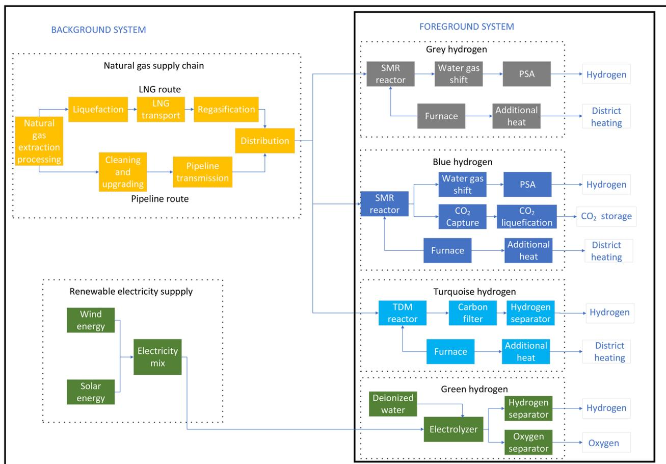
Fig. 2 System boundary conditions for all systems.
