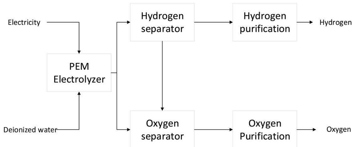
Fig. 5 Overview of green hydrogen (PEM electrolyzer) production (modified from Hermesmann & Müller, 2022).<sup>13,28</sup>
