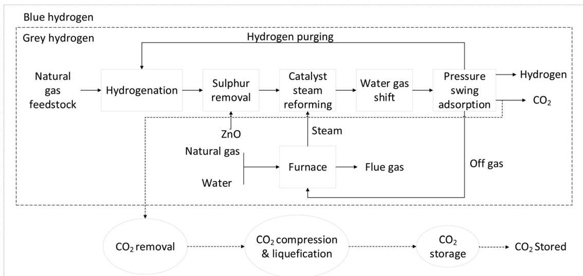
Fig. 3 Grey hydrogen (SMR) and blue hydrogen (SMR-CCS) production (modified from Petrescu *et al.*, 2014).<sup>19</sup>
