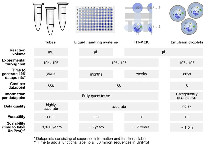
Fig. 1 Profiles of low to ultrahigh throughput experimentation systems (tubes, multiwell liquid handling systems, HT-MEK<sup>7</sup> and emulsion droplets<sup>8</sup>) that may be used as data generation tools for machine learning with their specific benefits and limitations.
