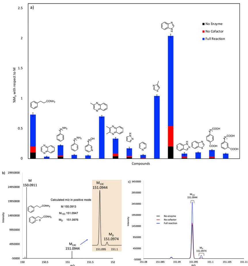
**Fig. 3** (a) Plot showing solvent deuterium incorporation in various substrates catalyzed by purified, holo-FDC. Mol% deuterium incorporations ( $\% M_D$ ) are shown relative to molecular ion ( $M$ ) peak for each compound. (b) Mass spectrum showing the calculated and experimental  $M$ ,  $M_{13C}$  and  $M_D$  peaks for 3-phenylpropanamide substrate. (c) Mass spectra for 3-phenylpropanamide of the experimental reaction, no enzyme, and no cofactor controls overlaid for comparison.
