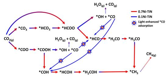
Proposed reaction mechanism over 0.7Ni-TiN and 0.1Ni-TiN
