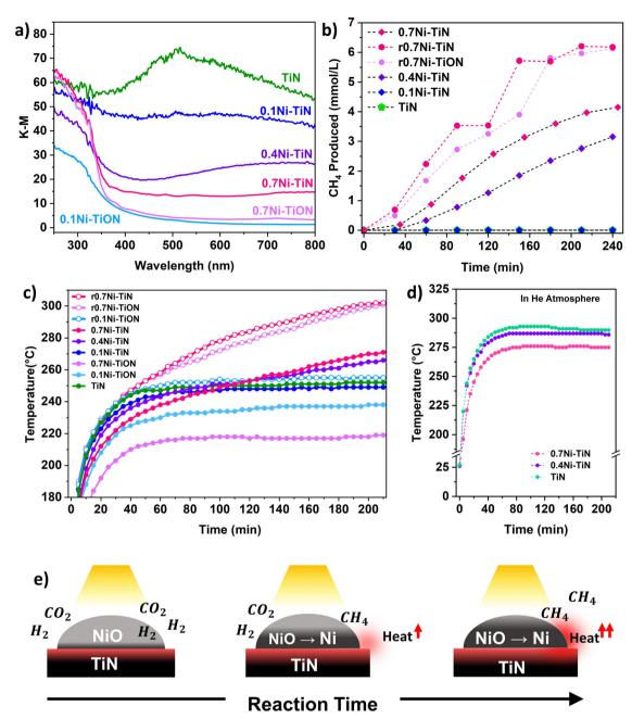
Fig. 2 (a) UV-vis absorption spectra for neat TiN, 0.1Ni-TiN, 0.4Ni-TiN, 0.7Ni-TiN and oxidised controls (0.1Ni-TiON, 0.7Ni-TiON); (b) photothermal CH<sub>4</sub> production by the various samples; (c) corresponding temperature profiles under photothermal conditions (Xe lamp at 20A setting); (d) xNi-TiN temperature profiles under inert He atmosphere (~80 kPa); (e) proposed photothermally-driven in situ Ni reduction mechanism.
