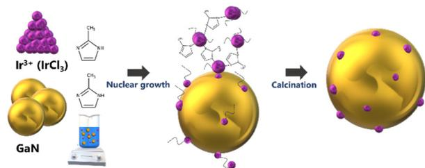
Fig. 1 Schematic diagram of the synthesis process for the nanocluster Ir<sup>3+</sup>/GaN catalyst.
