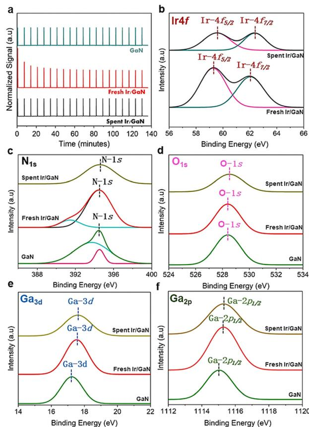
Fig. 3 (a) CO pulse chemisorption profiles of the GaN, fresh and spent Ir/GaN catalysts. (b) High-resolution XPS spectra of the  $\text{Ir}_{4f}$  and fresh and spent Ir/GaN catalysts. (c) XPS spectral surveys of  $\text{N}_{1s}$ . (d) XPS spectral surveys of  $\text{O}_{1s}$ . (e) XPS spectral surveys of  $\text{Ga}_{3d}$ . (f) XPS spectral surveys of  $\text{Ga}_{2p}$ .
