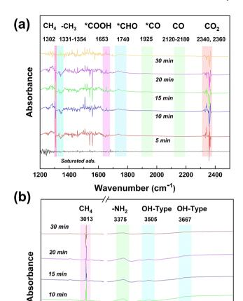
Fig. 12 In situ DRIFTS spectra of chemical substances and intermediates in the photocatalytic  $CH_4$  reforming process by  $CdS/TiO_2@NH_2-MIL-101$  catalysts.
