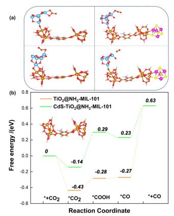
Fig. 10 Energy barrier change diagram of  $CO_2$  to CO photocatalyzed by the MOF-based composite catalysts.
