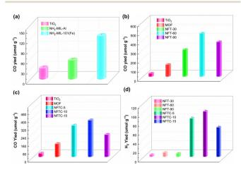
Fig. 6 CO and H<sub>2</sub> yield rates of various samples (4 h).
