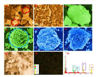
Fig. 2 (a)-(f) SEM images of catalysts; (g)-(i) EDX mapping images of NFTC-10.
