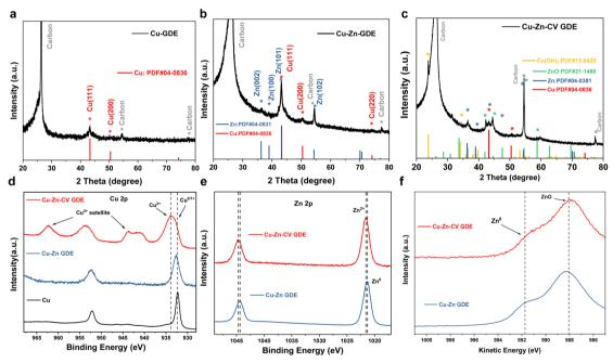
Fig. 3 XRD patterns of (a) Cu-GDE, (b) Cu-Zn-GDE and (c) Cu-Zn-CV-GDE catalysts. (d) Cu 2p XPS spectra of Cu-GDE, Cu-Zn-GDE and Cu-Zn-CV-GDE catalysts. GDE catalysts. (e) Corresponding Zn 2p XPS spectra of Cu-Zn-GDE and Cu-Zn-CV-GDE catalysts. (f) Zn LMM spectra of Cu-Zn-GDE and Cu-Zn-CV-GDE catalysts
