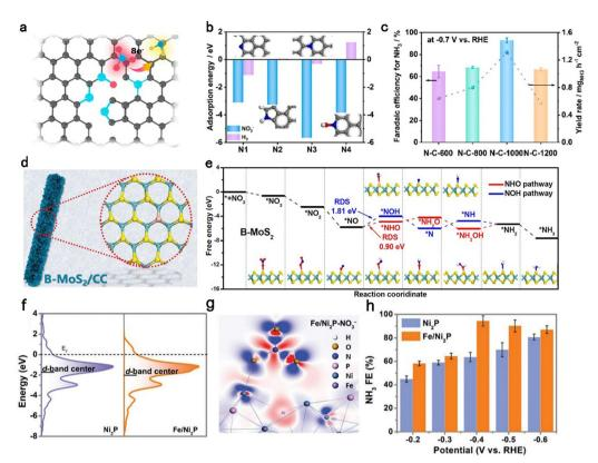
Fig. 4 Doping strategy. (a) Schematic of the structure of the N–C-1000 catalyst. (b) The adsorption energy of  $NO_3^-$  and hydrogen on pyridinic-N, pyrrolic-N, graphitic-N, and pyridinic-N-oxide moieties, respectively. (c) Faradaic efficiency and yield rate of  $NO_3^-$  for  $N-C-1000.^{33}$  Copyright 2023, Elsevier. (d) Schematic of  $NO_3^-$  (e) Free energy diagram of the nitrate reduction to ammonia on  $NO_3^-$  (h) Fe of  $NO_3$
