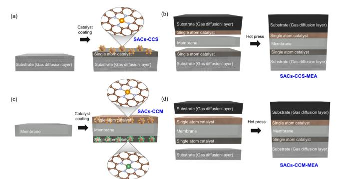
Schematic of (a) SAC-CCS-MEA and (b) MEA fabrication by hot pressing. (c) Schematic of the SAC-CCM-MEA and (d) MEA fabrication.
