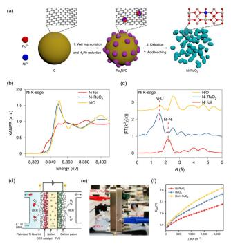
Fig. 11 (a) Schematic illustration of synthetic process of Ni-RuO2. The normalized (b) XANES and (c) EXAFS spectra of NiO, Ni foil, and Ni-RuO<sub>2</sub>. (d) Schematic and (e) digital photograph of PEMWE device. (f) I-V curves of PEMWE device using Ni-RuO<sub>2</sub>, RuO<sub>2</sub>, and Com-RuO<sub>2</sub> as OER catalyst and commercial Pt/C as HER catalyst. Reproduced with permission from ref. 195. Copyright 2023. Springer Nature.
