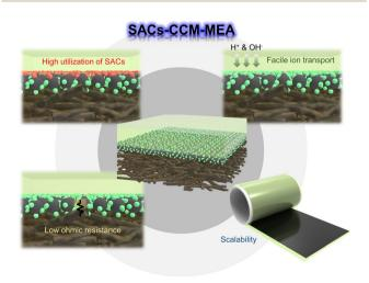
Schematic of the advantages of CCM-MEA with single atom Fig. 14 catalysts
