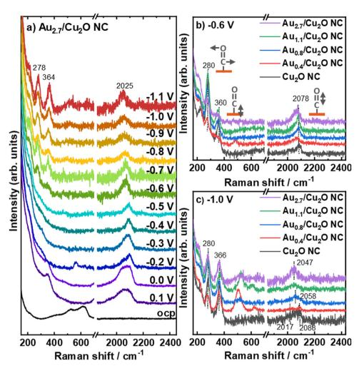
Fig. 6 Operando SERS of (a) Au<sub>2.7</sub>/Cu<sub>2</sub>O NC under potential dependence and of all Au-Cu<sub>2</sub>O catalysts at (b) -0.6 V and (c) -1.1 V in CO<sub>2</sub>-saturated 0.1 M KHCO<sub>3</sub>. Data for the Cu<sub>2</sub>O NC are redrawn from ref. 9
