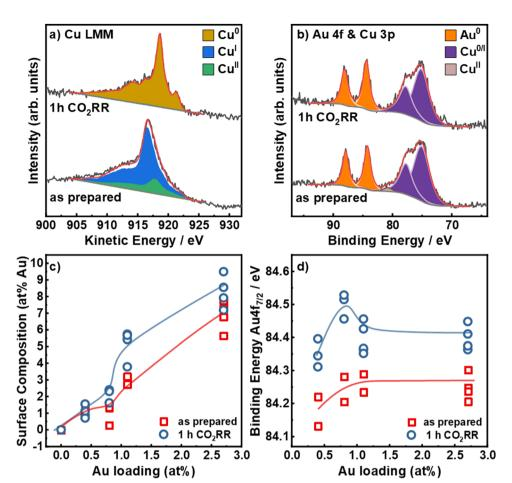
Fig. 3 Quasi in situ XPS spectra for the Au<sub>2.7</sub>/Cu<sub>2</sub>O NCs: (a) Cu LMM Auger and (b) Au 4f and Cu 3p in the as-prepared state and after 1 h CO<sub>2</sub>RR at -1.05 V vs. RHE in 0.1 M KHCO<sub>3</sub>. (c) Au: Cu ratio (at%) at the catalysts surface in the as prepared state and after CO<sub>2</sub>RR as a function of the nominal Au loading (determined by ICP-MS). (d) Binding Energies of the Au  $4f_{7/2}$  core level region in the as-prepared state and after 1 h  $CO_2RR$ .
