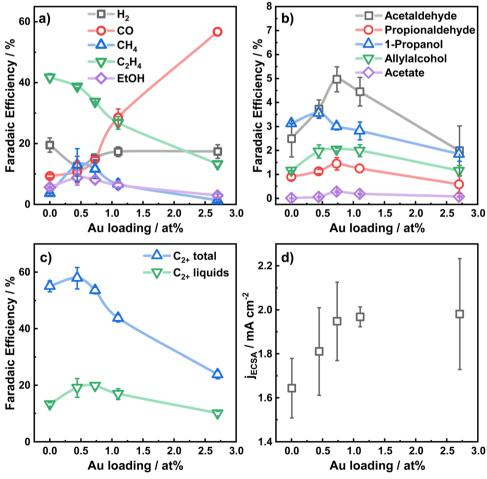
Fig. 2 Faradaic efficiencies at -1.07 V in 0.1 M KHCO $_3$  as a function of the Au NP loading for (a)  $H_2$ , CO, CH $_4$ , C $_2$ H $_4$ , (b) minor liquid products, (c) C $_2$ + total products, C<sub>2+</sub> liquid products; (d) Au-loading dependency of the current density normalized by the electrochemical surface area.
