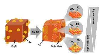
Fig. 7 Schematic illustration of the catalyst structure in the as-prepared state and during/after the  $\rm CO_2RR$ , with their corresponding main products. The triangles indicate the amount of Au loading favoring the different Au–Cu atomic structures/redistributions.
