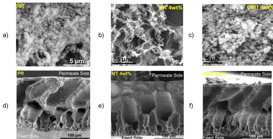
Fig. 2 Surface SEM images (magnification  $\times 8500$ ) of a) pristine PVDF, and MMMs having b) 4 wt% of MT, and c) 4 wt% of OMT; and membrane cross-sections (magnification  $\times 600$ ) of d) pristine PVDF, and MMMs of e) MT and f) OMT at 4 wt% both of each.
