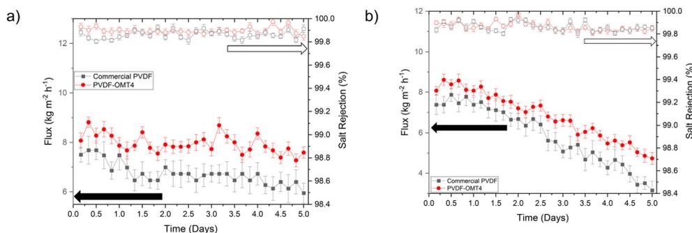
**Fig. 7** Long-term stability test of commercial PVDF (black lines) and PVDF-OMT4 wt% (red lines) membranes for permeate flux and salt rejection in presence of only a) NaCl and b) NaCl with HA to promote scaling phenomena. Full and empty symbols represent the membrane flux (kg m<sup>-2</sup> h<sup>-1</sup>) and salt rejection (%), respectively. Error bars represent standard deviations from three samples (or five in the case of the porosity).
