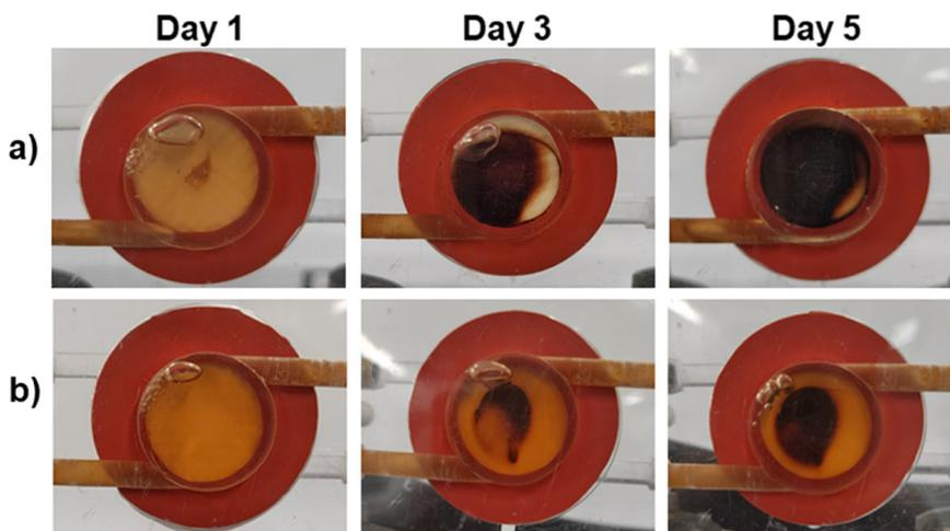
Fig. 8 Humic acid accumulation at the surface of the membrane after day 1, 3 and 5, for (a) commercial PVDF, and (b) OMT4 membranes (from top to bottom).
