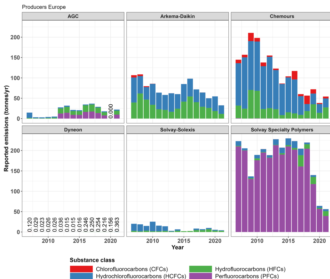
Fig. 2 Reported fluorinated gas emissions to the E-PRTR by European fluoropolymer producers. Note the missing data for AGC in 2020 and that there are some reported emissions for Dyneon but, as they are much lower than for other producers, the bars are barely visible and therefore the sum of emissions are shown per year.
