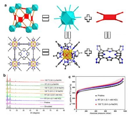
Fig. 3 (a) Structural analysis of PCN-601. (b) PXRD patterns for simulated, pristine PCN-601, and PCN-601 samples treated under different conditions. (c) N<sub>2</sub> adsorption/desorption isotherms at 77 K of pristine PCN-601 and acid and base treated PCN-601 samples. Reproduced from ref. 88. Copyright 2022 ACS.
