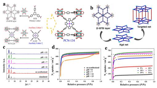
Fig. 6 Design of mixed-linker Zr-MOFs: (a) and (b) PCN-134 and PCN-224 formed by the 6-connected Zr<sub>6</sub> cluster and TCPP. (c) The XRD patterns and (d) the N2 isotherms after immersion in aqueous solutions with different pH values at room temperature for 24 h. (e) Effects of TCPP defects of the PCN-134 system on N<sub>2</sub> uptake measured at 77 K. Reproduced from ref. 98. Copyright 2022 ACS.
