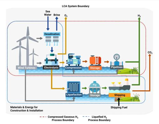
Fig. 9 The system boundary and process boundaries for compressed gaseous hydrogen pipelines and liquefied hydrogen shipping pathways used for the cradle-to-gate life cycle assessment of hydrogen produced offshore. This figure was designed using images from https://Flaticon.com.
