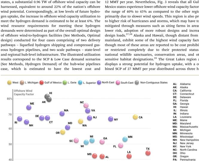
Fig. 3 Annual offshore wind capacity factors vs. serviceable hydrogen consumption potential for coastal states in the US, grouped by hubs to illustrate variations within and among the different regional hubs. Most coastal states have high quality wind resources, but concentration of multiple states with high CF and small demands in North-East and large intra-regional variations in South-East and West regions highlight potential for centralization through hub formation
